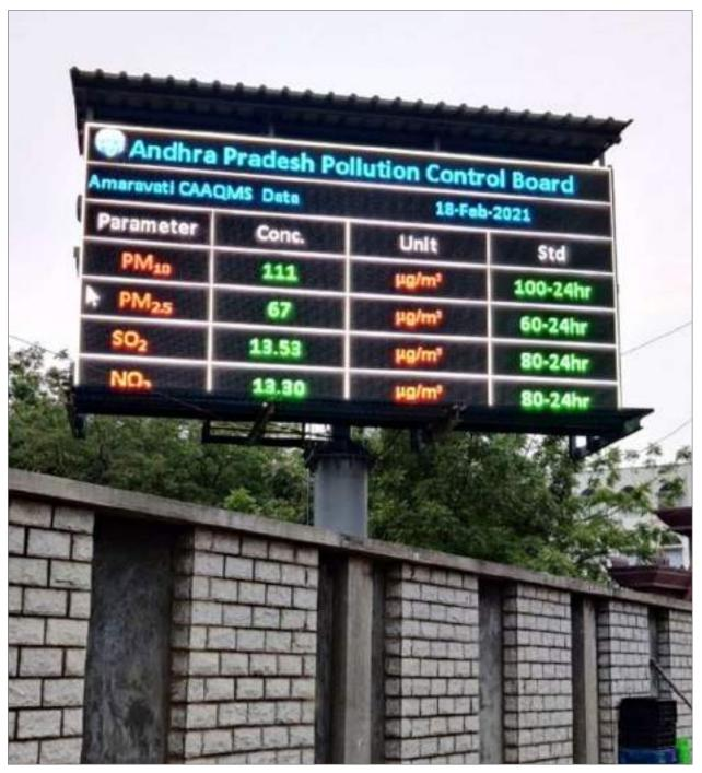
Image 4.28: View of Continuous Ambient Air Quality Monitoring Station near Polyclinic Road
